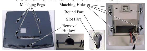
Align the matching pegs on the back of the main unit against one of the two sets of matching holes on the stand base. It is recommended that the terminal be hooked onto the lower set of holes for better stability. First aim the matching pegs
